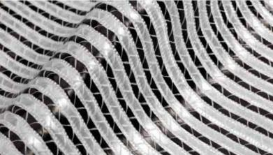
The flexibility of the fibres within the fabric structure ensures the outstanding drapability. For this reason, DRAPFIX can be perfectly applied to any complex shape as a local reinforcement.
