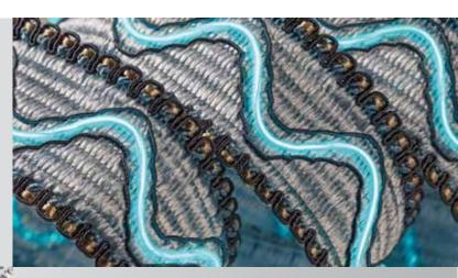
For technical applications, we offer a variety of textile-based solutions for humidity, temperature, pressure, load and deformation assessment. Most of these are implemented using conductive and semi-conductive materials.
