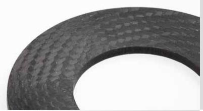
Spiral ribbons have outstanding robustness and dimentional stability owing to the return weft process and fibre orientation following the load paths.
