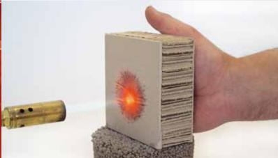
The specially produced glass-fibre textile is laminated with the flamme-resistive resin by Keraguss that hardens at room temperature. The harderning process can be speeded up by applying higher temperatures.
